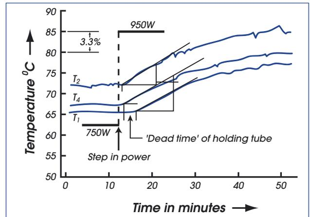
Fig 1: Open-loop temperature responses to a step in change (in power). Use of a 'reaction curve' method to obtain optimum P+I+D settings for a process temperature ( $T_1$ ,  $T_2$  and  $T_4$ ) to control the power to the heater vessel.
