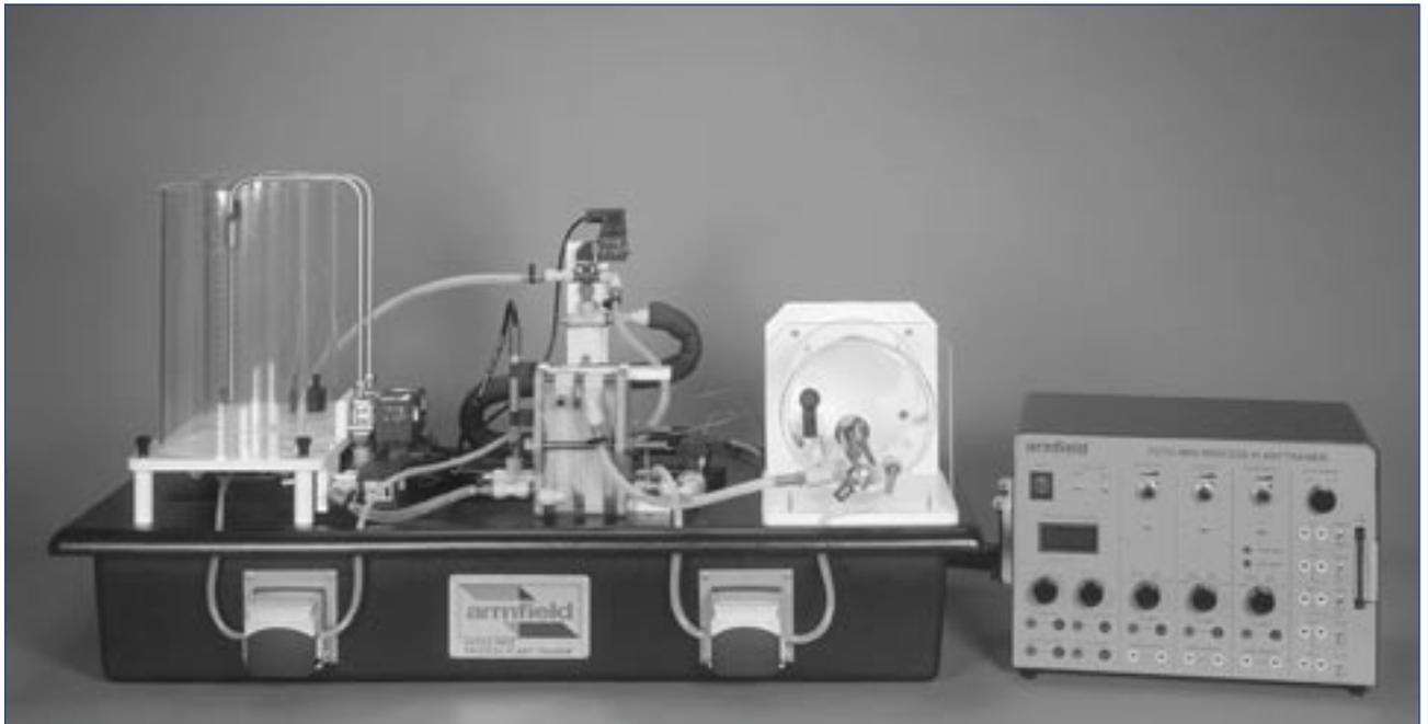
*The Armfield Process Plant Trainer can be used to demonstrate a complete range of process control methods and strategies. Manual control, single feedback loops, through to sophisticated cascade loops and distributed supervisory control of the whole process by a remotely located computer can be demonstrated. The system is a miniature replication of a true production process. The student is presented with real process control problems, with realistic dynamic behaviour and instabilities.*
