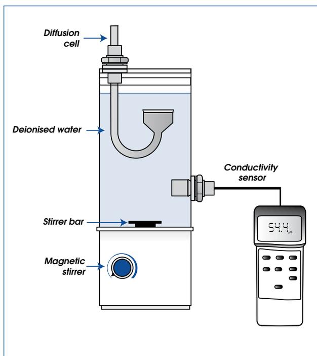
CERb: Liquid diffusion coefficients apparatus - equipment set-up
