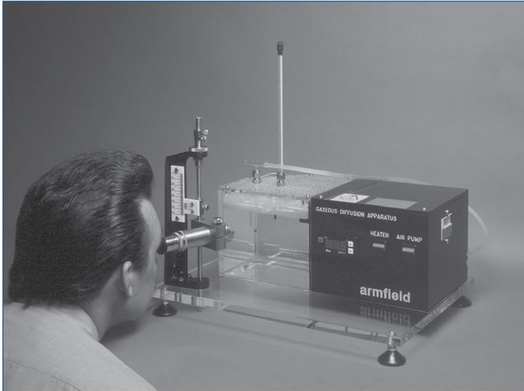
CERa Gaseous Diffusion Coefficients Apparatus
