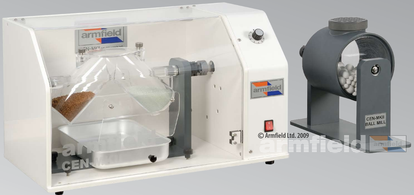
CEN-MkII-11 Shown with V blender installed and ball mill
