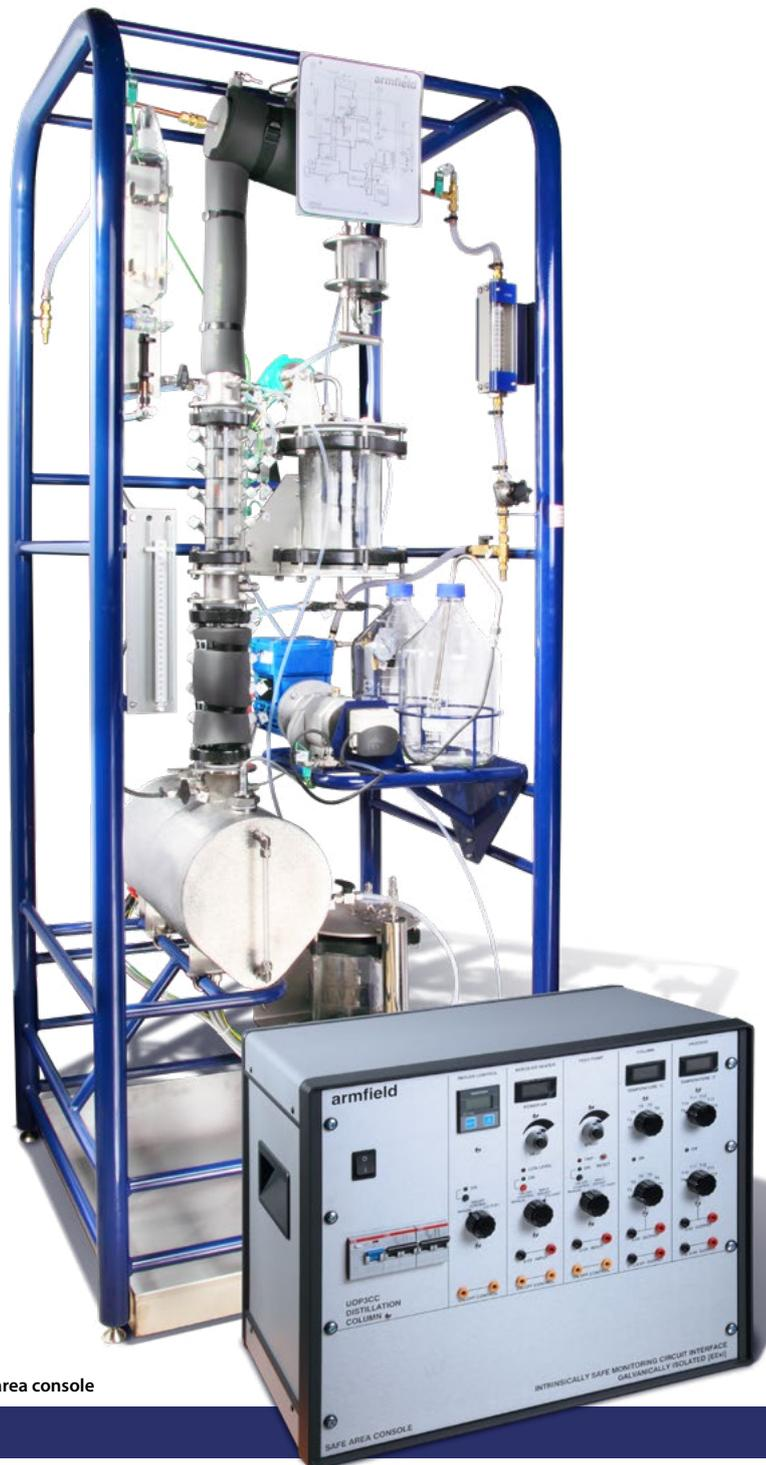
Above right: Computer interfaced distillation column UOP3CC shown with safe area console
