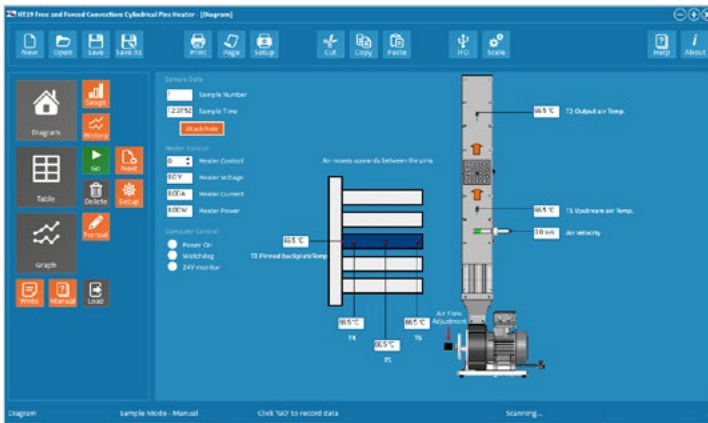
Typical mimic diagram showing the flat plate heated surface in the HT19
