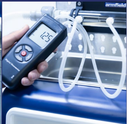
Supplied with digital manometer and thermometer
