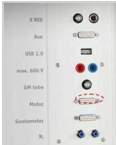
Fig. 3: Connector inside the experiment chamber
