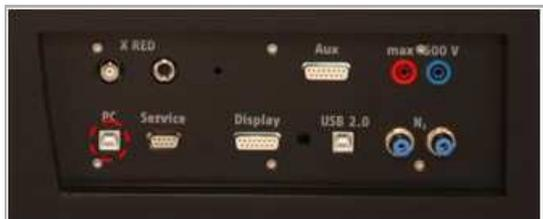
Fig. 2: Connection of the computer
