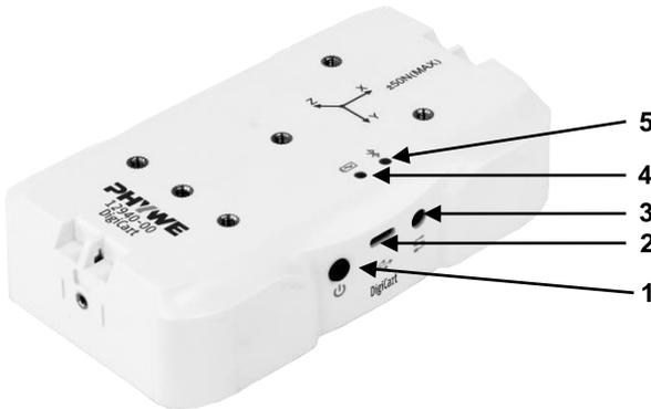
1. Power switch (press 3s to switch on)
