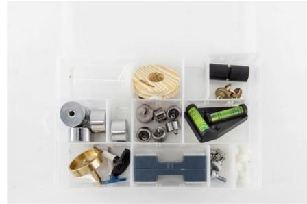
Accessory set A includes short screws, hook weights, weights, bucket, thread, spring, collision magnet, collision adhesive components, levelling instrument, screws, hand screw screws, etc.
