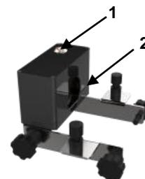
1. Push-button switch for triggering
